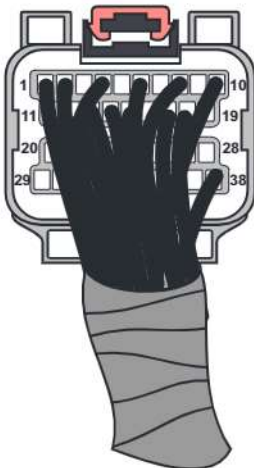
C4 Connector Wire Side View
