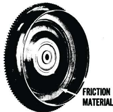
Fig. 7 — Lock-up friction material is bonded inside impeller front cover.
