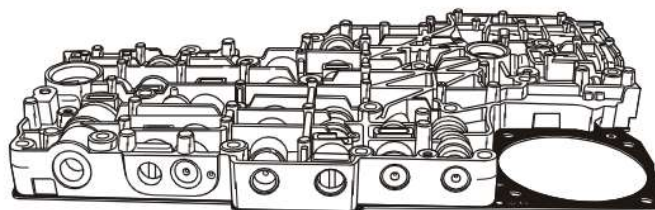
"5R55W/S" VALVE BODY ASSEMBLY
