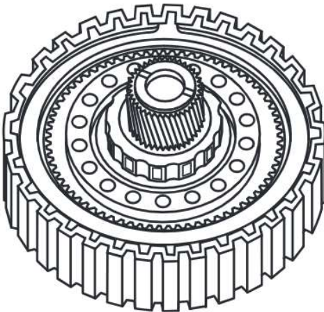
"STAMPED STEEL" COAST CLUTCH DRUM USED WITH 5.4L AND 6.8L "WITHOUT" PTO OPTION
