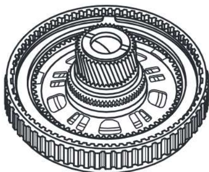
"CAST IRON" COAST CLUTCH DRUM USED WITH 5.4L AND 6.8L "WITHOUT" PTO OPTION
