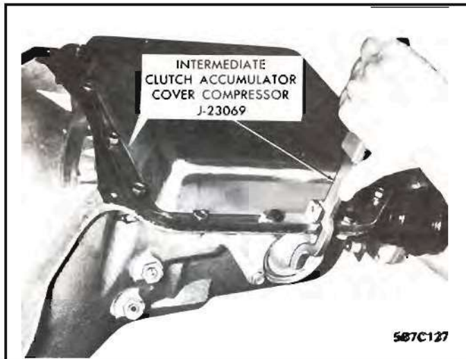
Figure 44 1-2 Accumulator Cover Removal
