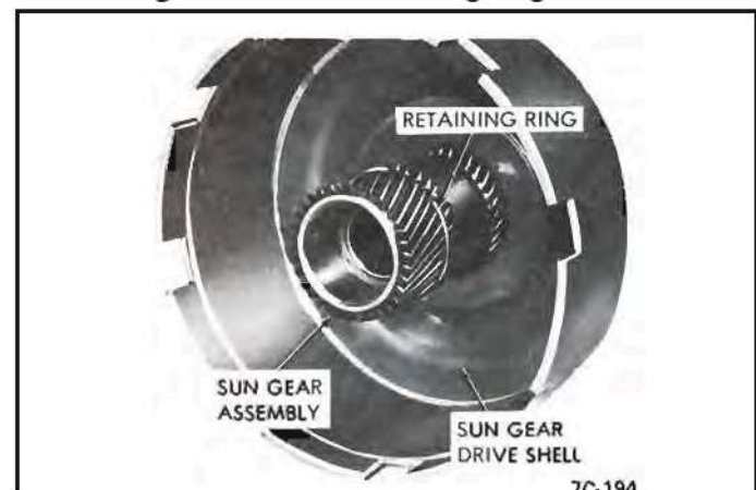
Figure 71 Front Retaining Ring Removal
