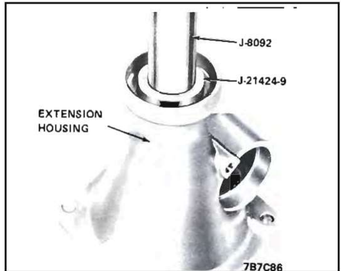
Figure 124 Extension Housing Bushing Installation
