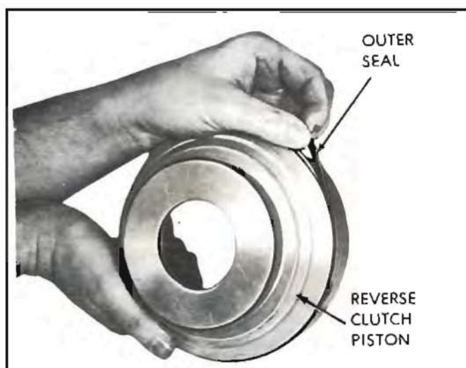
Figure 78 Outer Seal Installation
