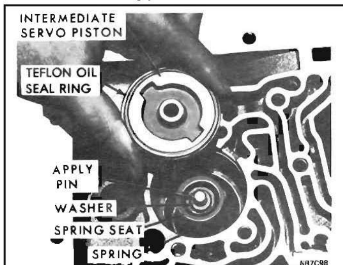
Figure 28 Intermediate Servo Assembly
